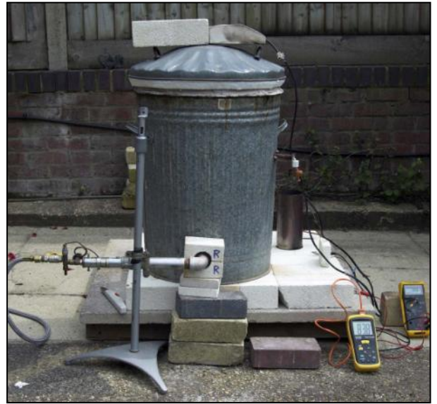
My dust-bin kiln, with the sensor mounted above the flue, the burner's air ports closed off, and the kiln's burner port blocked off with two shaped fire bricks. The meter on the far right shows the sensor output, whilst the other gives the current temperature.
