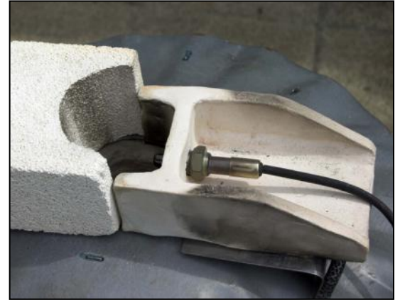
My sensor mounting, sitting above the flue port. The fire brick on the left is to ensure that the flue gases pass the sensor even if there is a side breeze. The wires are connected to an electrical volt meter.
