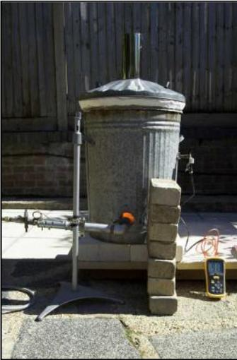
My initial gas kiln, having been constructed from a foldaway dog crate, rescued from the local council recycling centre, and insulated with 2" of ceramic fibre, was limited by the need to run it in fair weather, and also the life of the ceramic fibre. It consumed a lot of gas if I only wanted to test fire one or two small pieces, so then I built a 'dust-bin' kiln, also rescued from the local re-cycling centre!
